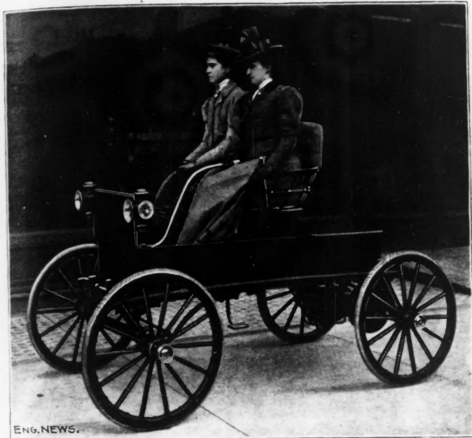
FIG. 1.—LIGHT BUGGY OPERATED BY STORAGE BATTERIES. FISCHER EQUIPMENT CO., MAKERS.
