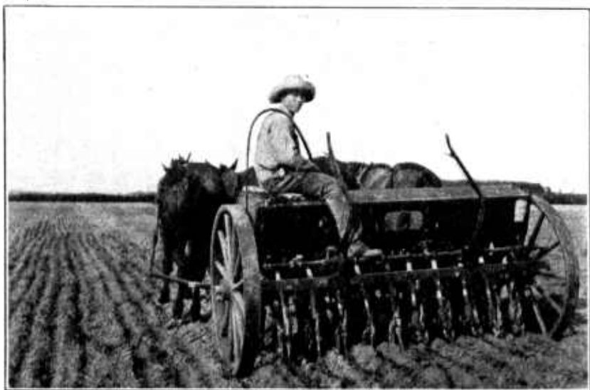
FIG. 5.—The ordinary grain drill may be used for sowing either in rows or in close drills
