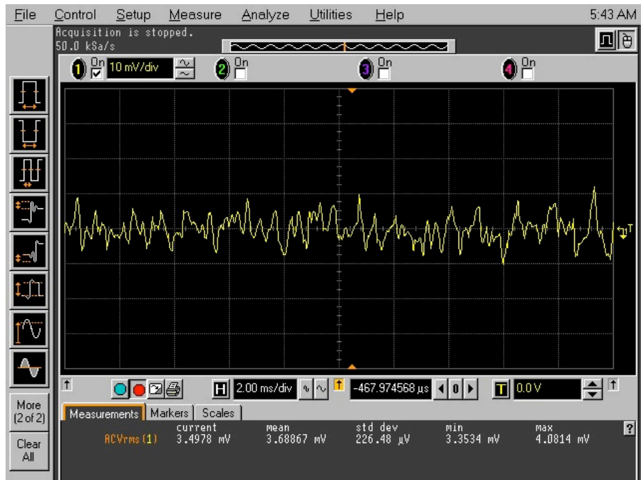
Figure 36. The noise floor with short leads showed a variance lower than the noise floor with long leads.
