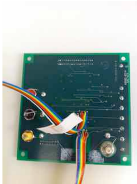
Figure 27. The soldered underside of the MS3110 evaluation board is shown here.
