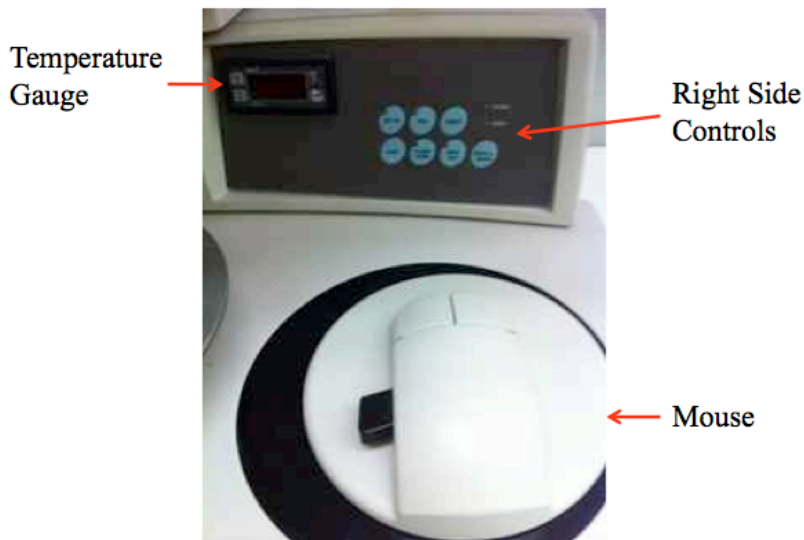
Figure 20. The wire bonder right control panel is shown here with various components depicted.
