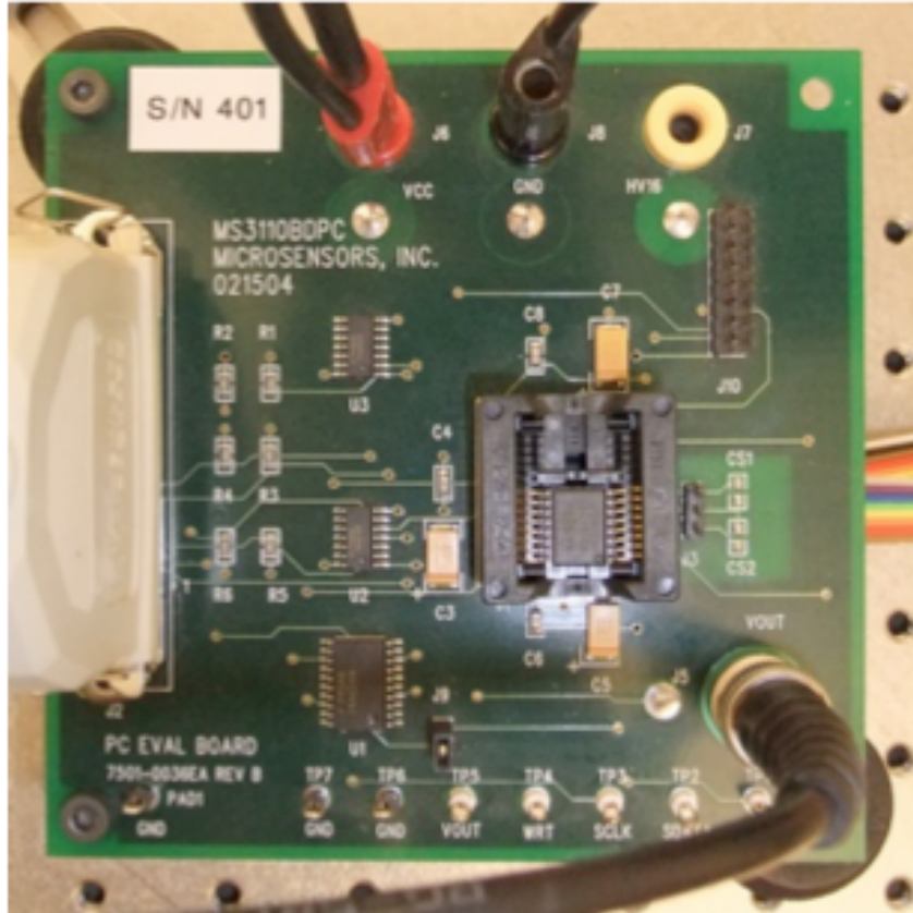
Figure 11. Here the interconnects of the MS3110 evaluation board are shown (From [12]).
