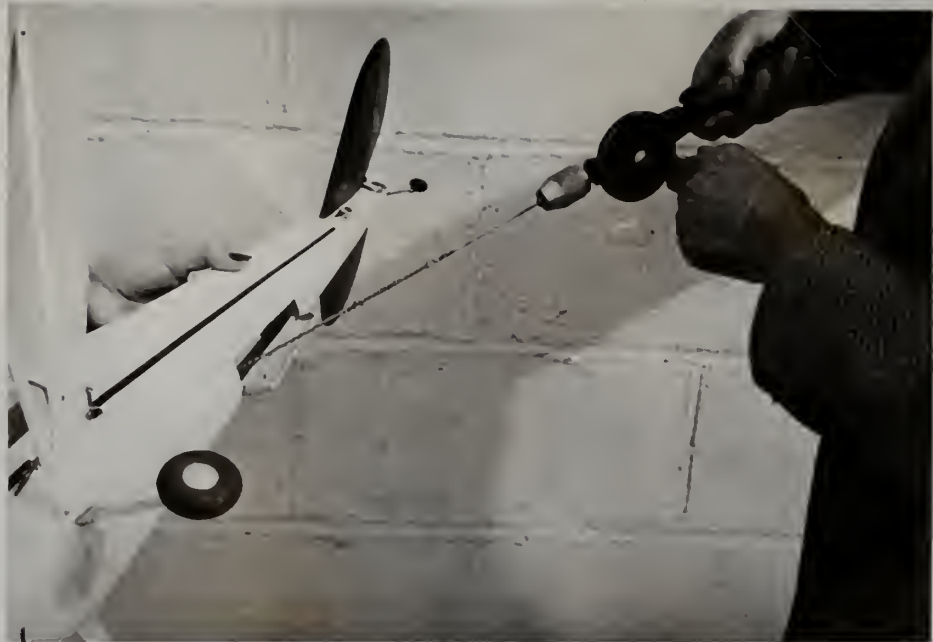
FIGURE 4e. - SHOWING METHOD OF WINDING RUBBER MOTOR OF ELEVATOR PULSING MECHANISM
