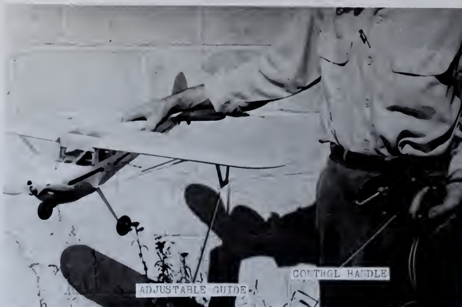
FIGURE 4d. - SHOWING PRIMARY CONTROL WIRES AND CONTROL HANDLE
