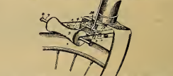
Claim.—A bicycle brake, consisting of a suitable frame, adjustable front fork with shoulders intermediate their ends and having a threaded connection with the brake-frame and adapted to engage sockets in the fork of the machine, a brake-shoe attached to said frame, and means for adjusting the brake-fram, substantially as described.
