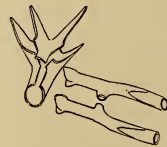
Rambler Crank-Hanger and Dished Rear Fork.
