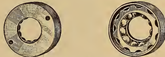
Ball Cups in the Bottom Bracket of the 1897 Gendron and Reliance Bicycles.
