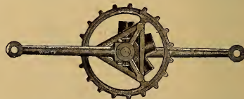
The Weston-Mott Co.'s New Crank Hanger and Sprocket.
