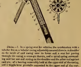
Claim-1. In a spring-steel for a vehicle, the combination with a tubular frame, a tubular casing adjustably secured, in a shoulder on the inside of said casing near its lower end, and a spiral spring arranged through the casing, a cross-pin therein, and a spiral spring around said pin and one end resting on the shoulder and the other end against said pin, of a bearing member being at the opposite end of the casing, and a toggle lever pivotally connected to the upper end of the rear bar and so being arranged substantially as described.
