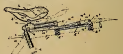
Claim.—The combination with the frame of a bicycle, of the saddle-pat, removably arranged in the diagonal seat frame, a fore or rear projecting front saddle-post, a clip connecting the forward portion of said tube or bar with the top tube of the frame, a sleeve on said tube or bar and adapted to slide thereon, the saddle carried by said sleeve, a lever fulcrumed on the top tube and in front of the clip, and an arm pivoted secured at one end to the sliding sleeve and at the other end to said lever, all said parts, substantially as and for the purpose described.
