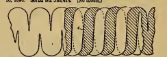
Claim.—A protector for pneumatic and other similar tires, composed of two bands having serpentine folds of any desired pitch, interwoven or interlocked substantially as herein described.
