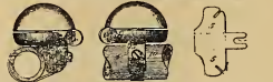
Claim.—In a clamp, the combination with a frame provided with parallel sides, and opposite key-holes, of a band-clip, means for securing it to the frame, a wire coil, and a winding-key at its free end, adapted to enter the key-hole in the frame, substantially as set forth.
