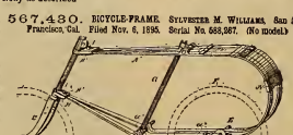
Claim-1. A bicycle frame composed of spring or elastic bars bent or curved upon themselves, having connections at their extremities with the stem of the front-wheel fork, connections at their rear lower portions with the axle of the rear wheel, an saddle-peg bar extending from the upper member of the front frame to the lower member thereof, and transverse journals on the upper and lower members of the frame to which said bar is connected whereby the frame is permitted to flex freely.
