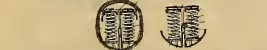
Claim.—As a new article of manufacture, in a spring-tire, the combination of a base-band that will encircle the rim of a wheel, and a tread of outer sheeted flexible plates, the ends of outer sheeted flexible plates.
