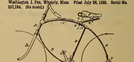
Claim-1. The combination of a bicycle-frame having a crank-shaft bearing end at its forward part an upper bar curved eccentrically to said bearing, the saddle-support 9 adjustably secured upon said eccentrically-curved bar, and the saddle adjustably secured on said saddle-support, whereby the height of the saddle relatively to the crank-shaft bearing may be adjusted without varying its relative position thereto from front to rear substantially as described.
