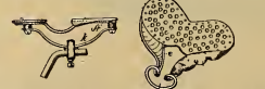
Claim.—A frame for a bicycle-saddle comprising two approximately elliptical loops, one forming the contour of the seat and the other the contour of the girth, and a contracted and depressed connection or bridge between the two loops, substantially as described.
