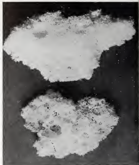
FOAMY structure of vacuum-dried milk (upper) is uniformly expanded to give good dispersibility. Caked spray-dried milk (lower) may not liquefy.
