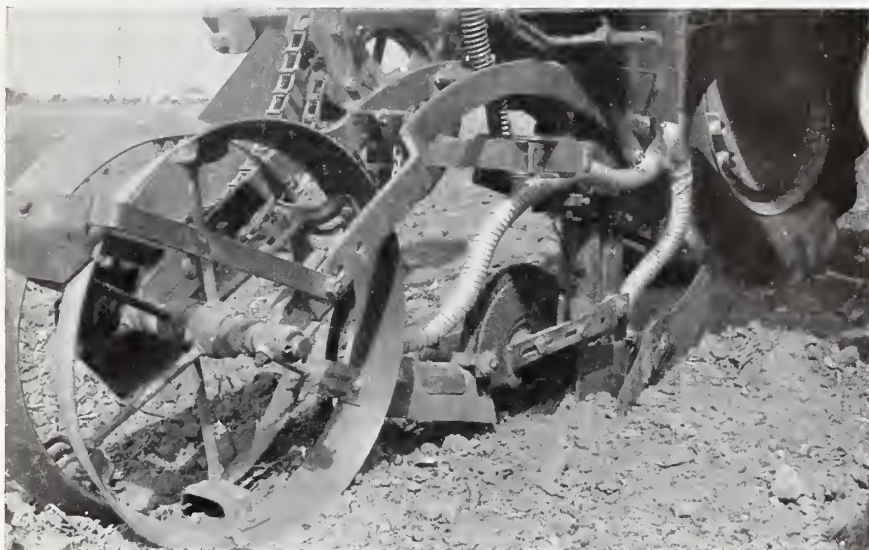
COVER DIRT , treated with fungicides (diagram), gives safe bed through which seedlings rise to surface. Attachments on planter (photograph) completely treat and place the furrow cover. Dust is delivered into covering soil through seed-drop tube (right) and by "Y" connection to rear of seed-firming wheel (center) to mix with upper soil and seed-row surface.
