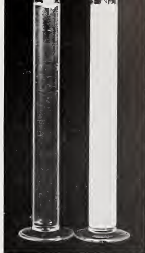
SELF-MIXING in ice water took 4 minutes for USDA milk. Most spray-dried whole milk (left) caked at surface.
