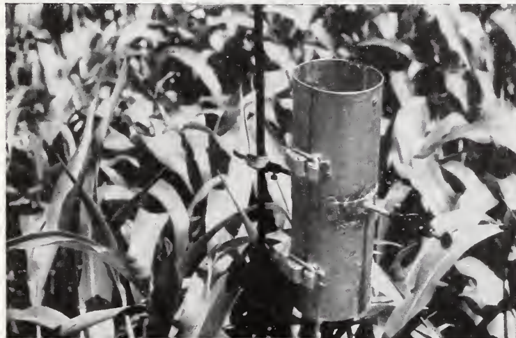
JOINED HALVES of cylindrical cup can be closed around head of sorghum plant, with stem extending through opening in bottom of cup (right). Tight seal is formed when halves are closed (above). Cup is 3 inches wide, 12 inches long, adjustable to any height for field or greenhouse work.
