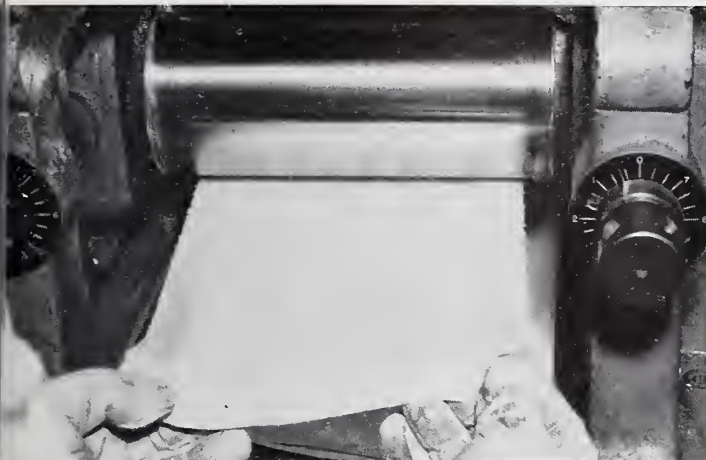
SHINY plastic sheet comes off rollers. Plastics with built-in animal fats are stronger, more flexible, and more durable in temperature extremes than plastics we've made heretofore.
