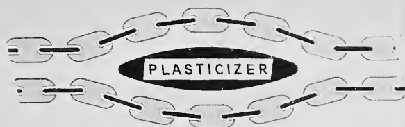
FATTY plasticizer fused or linked internally in the plastic's chemical structure (top) can't escape. But a plasticizer merely mixed with plastic (below) gets out.
