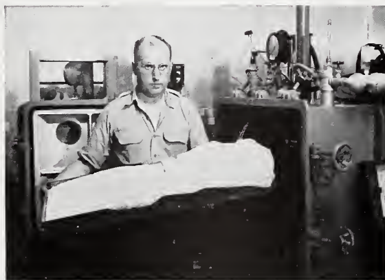
BATCH of whole-milk concentrate just out of vacuum dryer is greatly expanded and resemble mass of foam. This is one of 300 batches made by this process.
