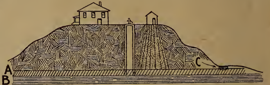
The water layer (A) is polluted by sewage coming through the porous soil (B) represents the impervious clay layer. The spring (C) will be contaminated, likewise the well. The well and spring are too near the source of pollution.
