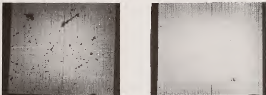
Figure 6. Scanning Auger, Cu 914 eV elemental maps, before (left view) and after (right view) laser quenching. The dark spots in the unirradiated elemental map correspond to the Fe-rich precipitates, which following resolidification from the melt are retained in solution with the Cu-Al FCC matrix.
