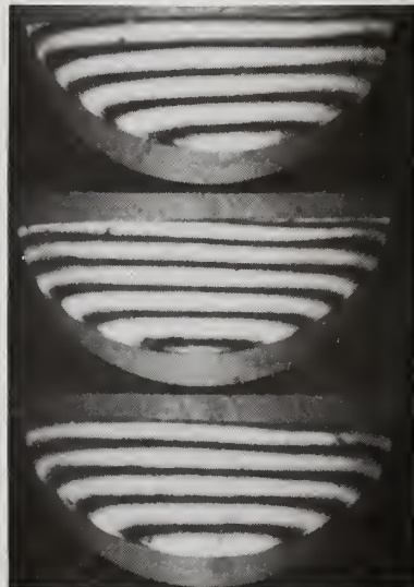
Figure 6. Interference fringes showing initial distortion and ultimate optical figure error of a ULE flat after thermal cycling to various temperatures up to 350°C. Both an air quench and a water quench were used. No ultimate thermally induced figure error can be observed for this material.
