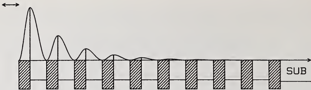
Figure 1. Time averaged square of the electric field strength for 248 nm radiation incident from the left on a 248 nm scandia/magnesium fluoride quarterwave stack. The arrows indicate the electric field intensities of the incident, reflected, and transmitted waves. The position of the layers is indicated below the field plot. The scandia layers are shaded.
