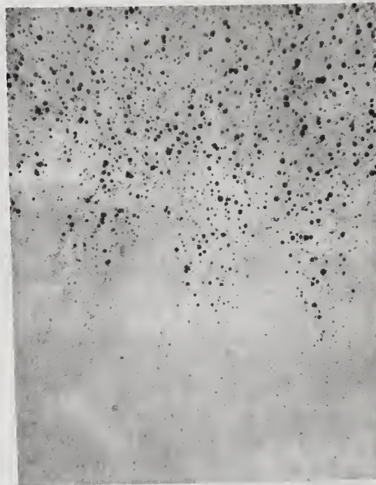
Fig. 6 Micrographs of copper mirror showing regions of substrate that were masked and unmasked from the carbyne vapor stream. Localized laser damage to carbyne coating occurs at carbon particulate sites.
