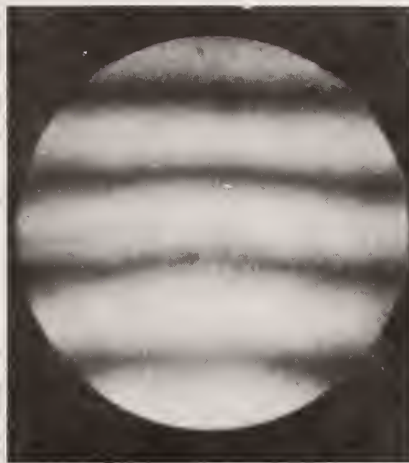
42 HOURS AFTER 250°C OVEN FRINGES HORIZONTAL
