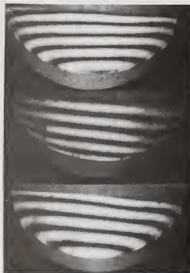
Figure 6. Interference fringes showing initial distortion and ultimate optical figure error of a ULE flat after thermal cycling to various temperatures up to 350°C. Both an air quench and a water quench were used. No ultimate thermally induced figure error can be observed for this material.
