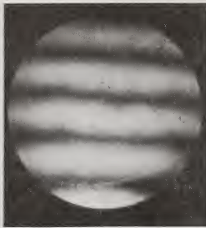
2 HOURS AFTER 50°C OVEN FRINGES HORIZONTAL
