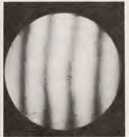
42 HOURS AFTER 250°C OVEN FRINGES VERTICAL
