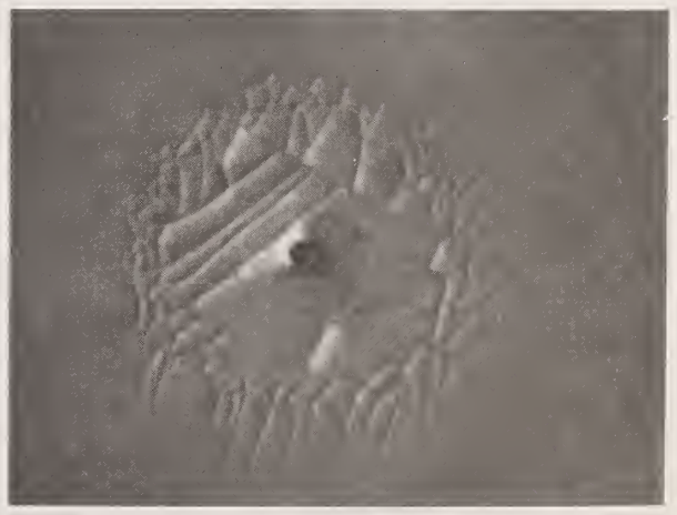
Figure 4. Laser damage at 1.06 μm on a polished, untreated NaCl surface.
