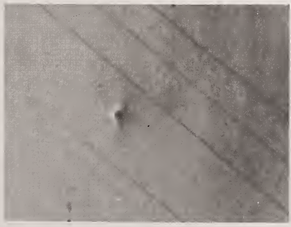
Figure 3. Laser damage at 1.06 μm on same surface shown in figure 2 after heat treatment. Note the marked change in damage morphology.
