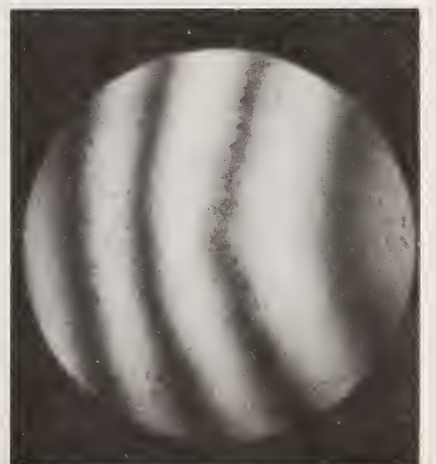
24 HOURS AFTER 300°C OVEN FRINGES VERTICAL
