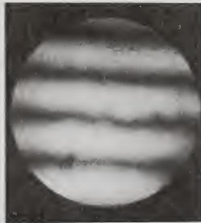
3 HOURS AFTER 150°C OVEN FRINGES HORIZONTAL
