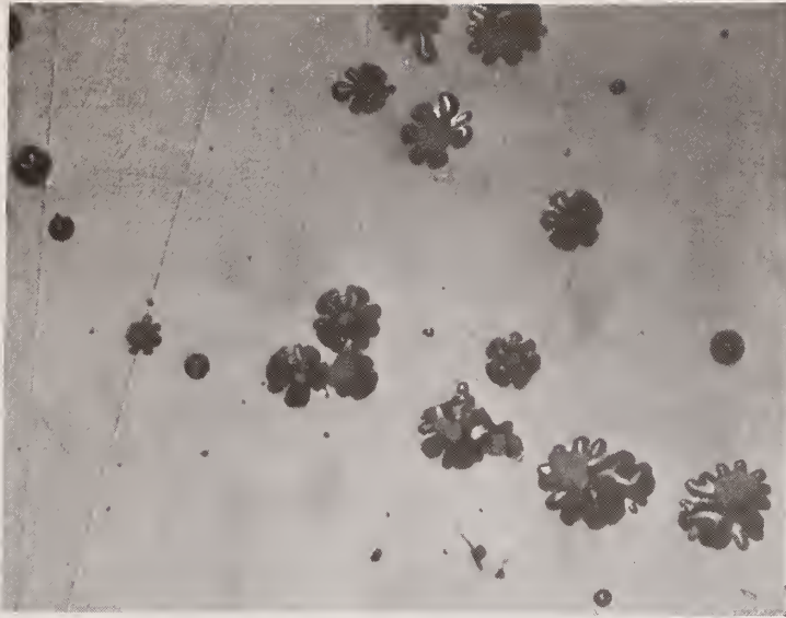
Fig. 4 Carbyne film on \text{CaF}_2 irradiated at 23\text{J}/\text{cm}^2 showing localized damage at carbon-bearing (black) spots. Magnification is 200:1.
