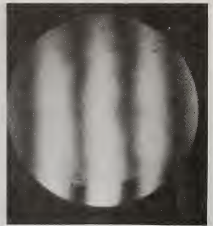
2 HOURS AFTER 50°C OVEN FRINGES VERTICAL
