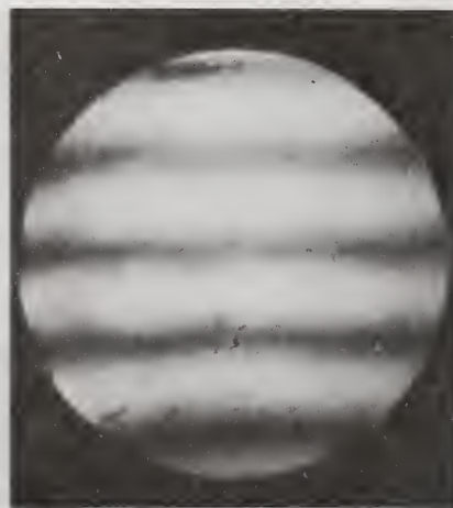
3 HOURS AFTER 100°C OVEN FRINGES HORIZONTAL
