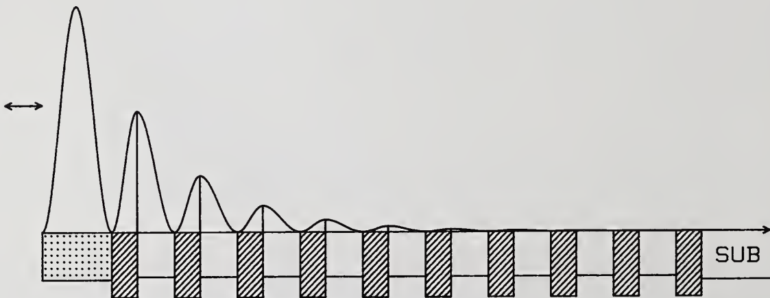
Figure 3. Similar to figure 1 for the scandia/magnesium fluoride reflector with halfwave silica overcoat. The silica layer is dotted.
