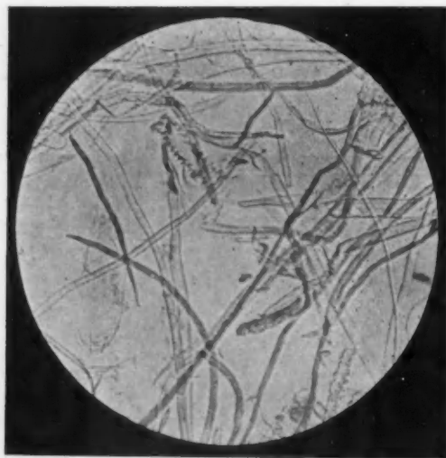
Fig. 7.—Elements of straw pulp mounted in glycerine. Magnification, 150 diameters. Note carefully the minute markings.
