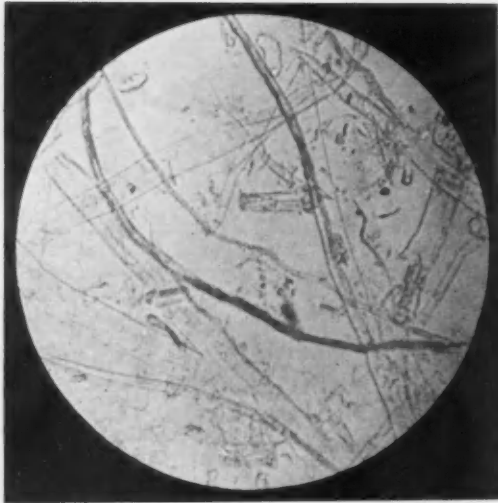
Fig. 8.—Elements of white lining of triplex board made on board machine. Magnification, 150 diameters. The lining was separated by gently boiling in weak caustic soda solution for two hours, then washing and carefully detaching lining from middle with forceps. The lining is said to consist of 85 per cent. sulphite pulp, with 15 per cent. bleached straw, heavily loaded with mineral and sized. The middles consisted of a mixture of broke paper and mechanical wood. The photograph shows distinctly the fine markings in the sulphite fibre, the mineral loading, and the characteristic cells, vessels and fibres of the straw.
