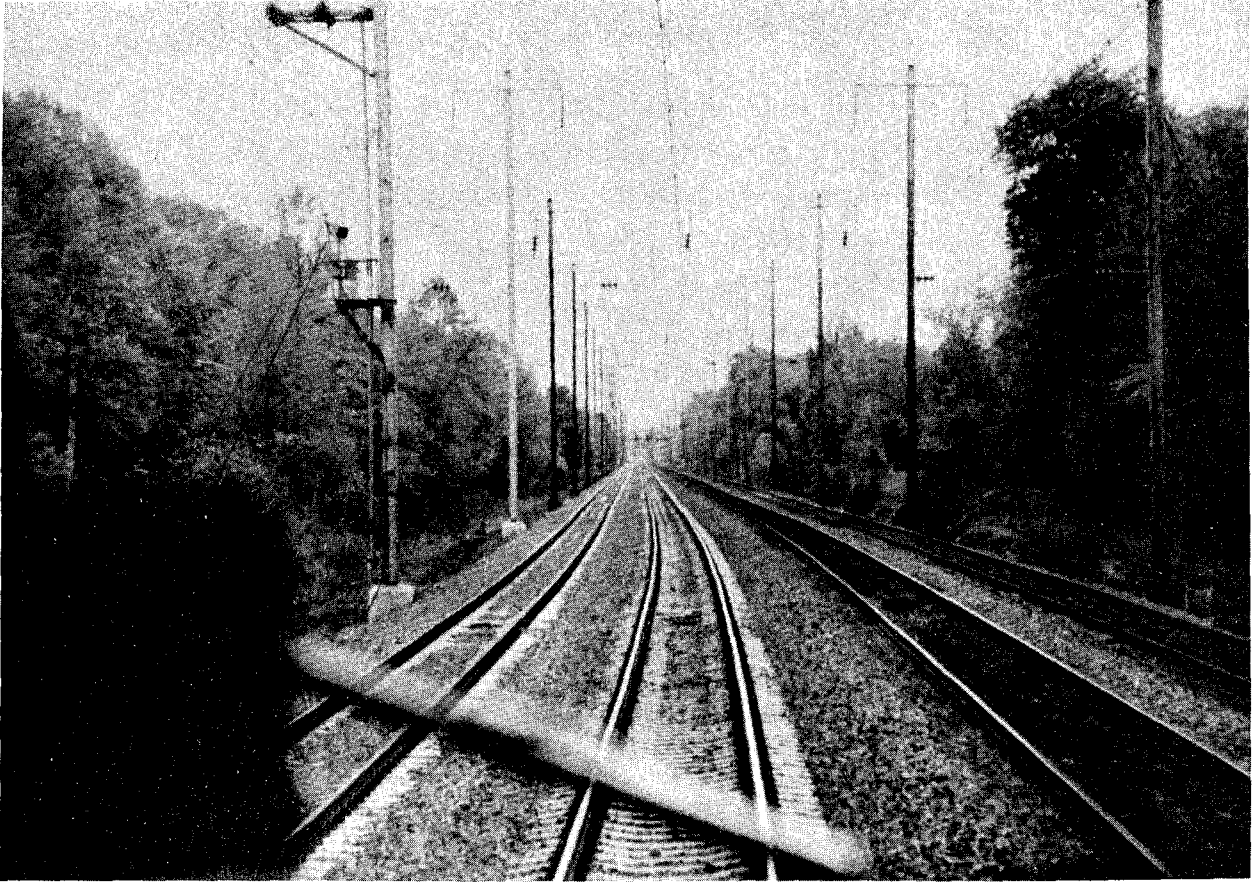
Figure 10. Code change point CS-806 as seen from a northbound train on track 2. The nearest catenary support poles mark the location of the code change point. The Gunpow home signals are in the distance.
