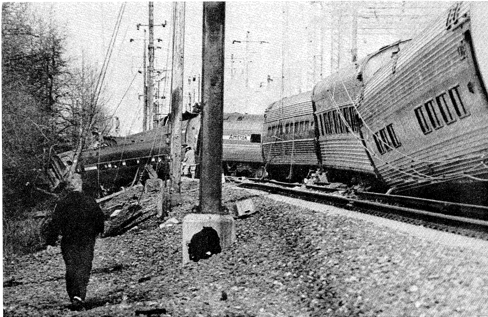
Figure 5. View from west side of the tracks facing north and showing derailed passenger cars of train 94. The car at the extreme right was the rear car of the train, and the car ahead of it was the second car from the rear. The poles in the middle held up the catenary wires. Fallen catenary and high-voltage transmission lines are on both sides of the poles.
