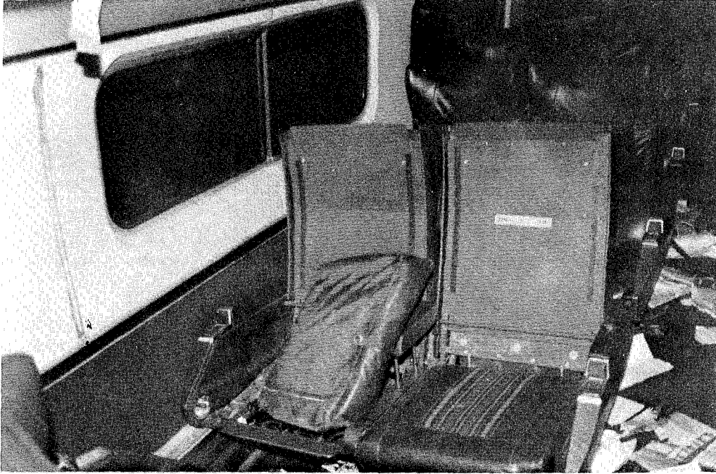
Figure 17. Missing seatback cushions and exposed sheetmetal seatback frames in a coach.
