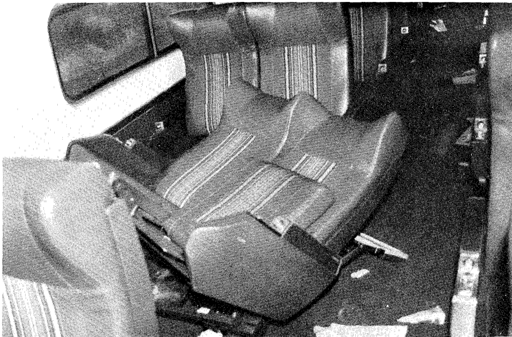
Figure 18. Seats separated from pedestals in the seventh car of train 94.
