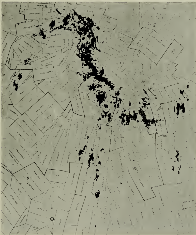
Map of claims showing the horizontal distribution of some of the proved bodies of ore. The Copper Queen Mine is represented in the upper left hand corner
