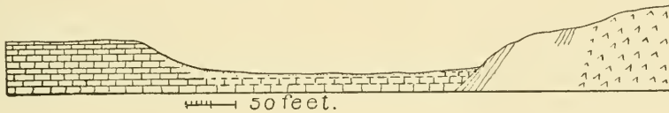
FIGURE 4.—Diagram to show the apparent relative positions of the limestone and crystallines east of Fort Hill. Horizontal and vertical scales equal.
