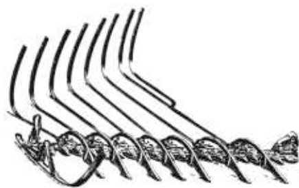
FIGURE 6.—Lifter guards and a wind-row attachment for mower to be used in harvesting lodged vetch.
