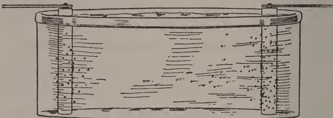
When an electric current is passed through water, oxygen and hydrogen come up in bubbles
