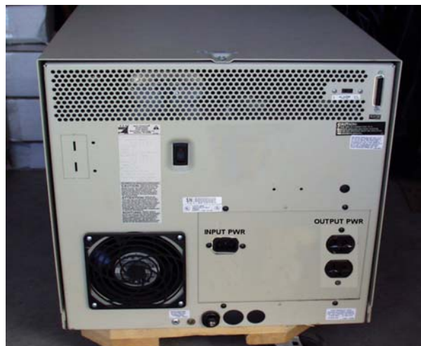
Figure 3.20: Rear Panel of the Modified UPS
