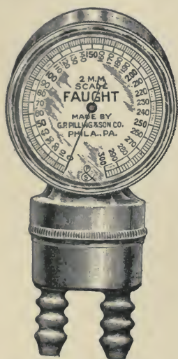
FIG. 8.—Faught pocket apparatus dial in detail.
