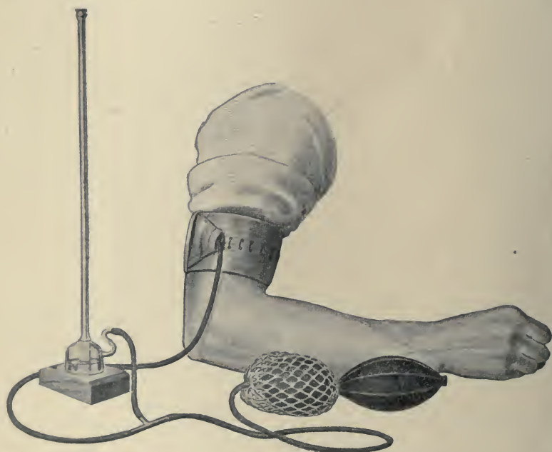
FIG. 3.—Cook's modification of the Riva-Rocci sphygmomanometer, showing narrow arm-band in place, with cautery bulb inflator.
