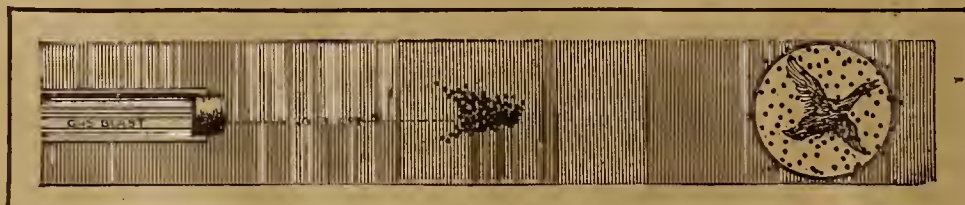
The Winchester system of wadding. The wadding expands evenly, sealing in the gas blast all the way to the muzzle, where the wadding is checked by the "choke" or constriction. The shot cluster travels ahead unbroken. Actual test target 320 pellets out of 431 or 74% of the shot charge (1 1/4 oz. of 7 1/2 chilled) inside a 30-inch circle at 40 yards.
