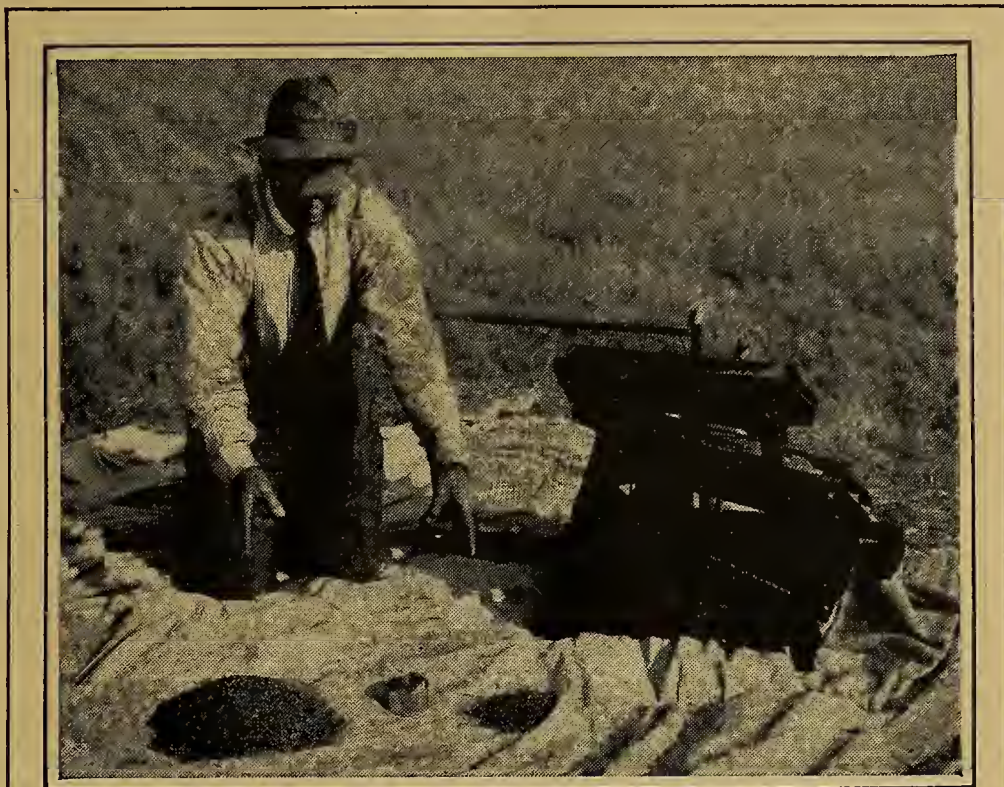
The large pile indicates the wastage found while threshing 2½ bushels. The small pile shows the wastage after the machine had been adjusted
