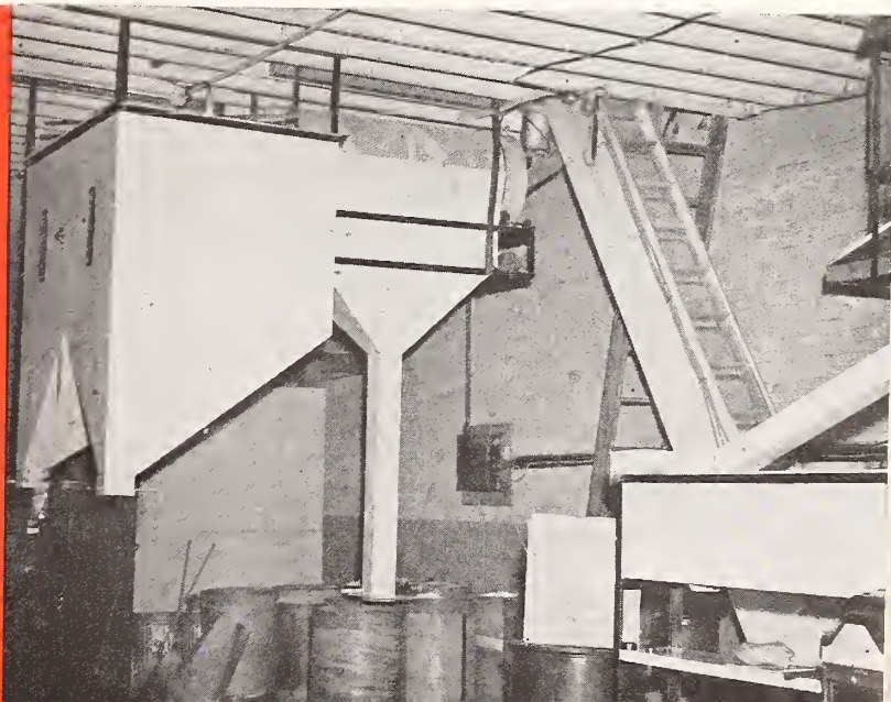
This elaborate corn popper fills the basement of the circuit's headquarters in Scranton. It can produce 1,400 pounds of popped and buttered corn a day.
