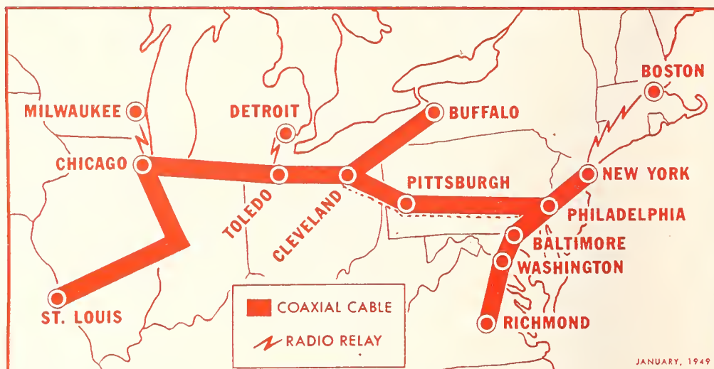
The Bell System coaxial cable and radio relay network as it will appear January 12, when, with the completion of the Philadelphia-Pittsburgh-Cleveland link, the first television program will go out over interconnected stations in the East and the Midwest.
