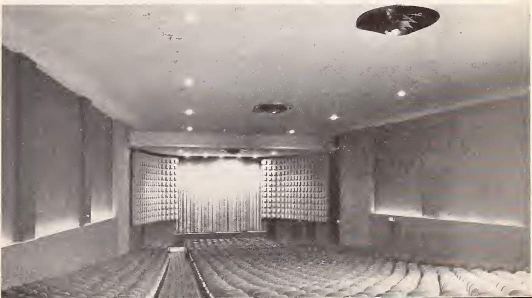
The auditorium — toward the stage (right) and toward the standee space (above), compared with the original plan and treatment in similar views. The side wall panels are covered in deep blue velour and are lighted by blue neon concealed in the top of the dado. The ceiling is acoustical plaster painted off-white. Seating is now on one floor.
