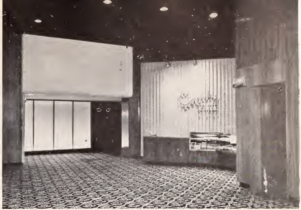
Comparative views of the foyer before and after remodeling. Above, looking toward the entranceway to the auditorium; below, looking into the lobby. Walls and facing of refreshment stand are of ribbon mahogany plywood, the plaster ceiling is painted blue-black.
