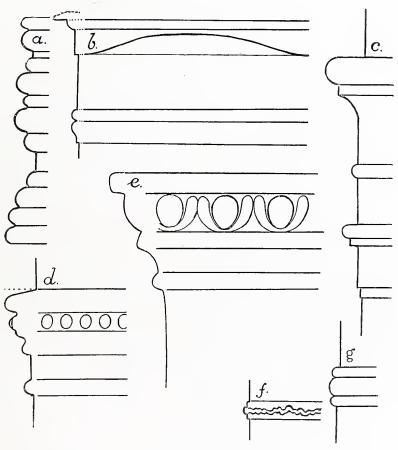
Fig. 149. Plaster Cornices and Mouldings.  $\times \frac{1}{2}$ .
