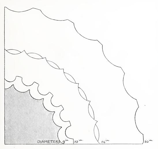
FIG. 135. Sections of Fluted Columns.  $\times \frac{1}{2}$ .
