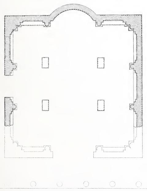
Fig. 28. Plan of the Temple, with suggested Restoration of a Portico.
