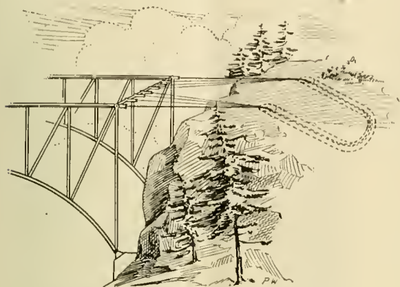
METHOD OF ANCHORING THE HALF-ARCHES.
