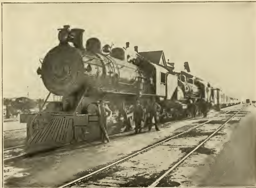
LOS ANGELES LIMITED, A. T. & S. F. THESE ENGINES BURN FUEL OIL.
