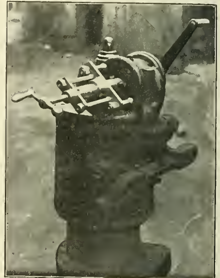
DEVICE FOR BORING VALVE BUSHINGS.
