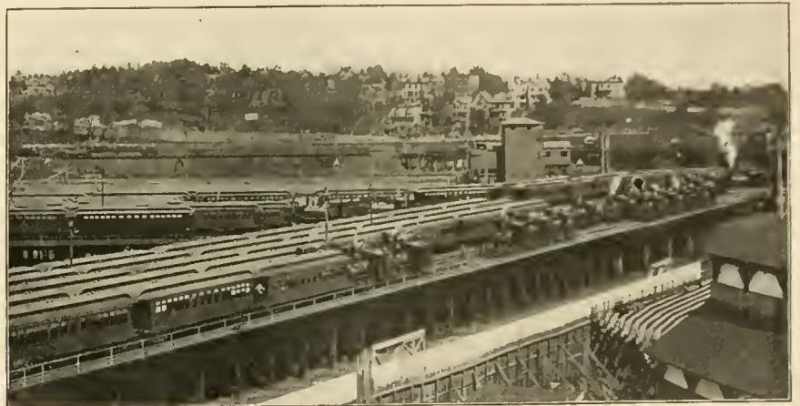
FORNEY ENGINES ON THE NEW YORK ELEVATED RAILROAD BEFORE THE ELECTRIC POWER WAS USED.
