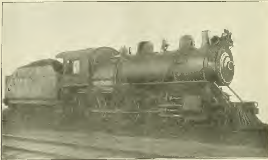
CULM BURNER, WHERE FIREMAN AND ENGINEER ARE TOGETHER IN ONE CAB. CANADIAN PACIFIC RAILWAY.
