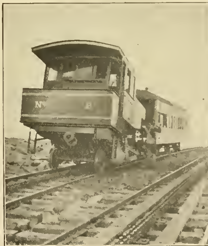
PIKE'S PEAK RAILWAY ENGINE, CAR AND PORTION OF TRACK SHOWING RACK RAIL.
