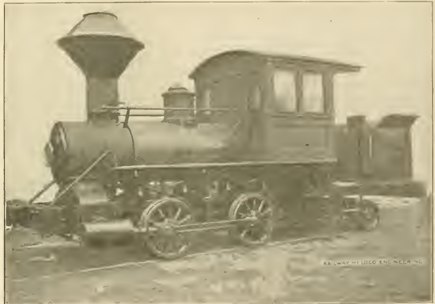
FIG. 30. ENGINE WITH OSCILLATING CYLINDER AND NO VALVE GEAR. (Described on page 539.)
