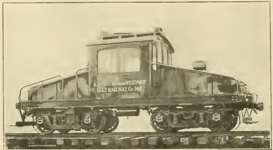
FIFTY-TON K. C. & W. ELECTRIC LOCOMOTIVE
