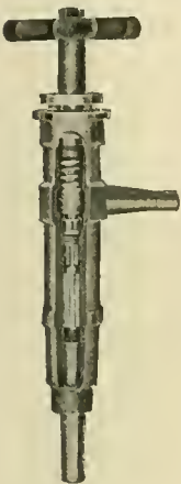
All Brass, extra heavy, with Cased Plug. For 250 lbs. pressure. Made with Draining Plug to prevent freezing.
