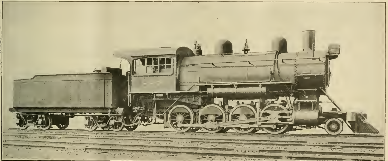
CONSOLIDATION OIL BURNER ON THE MEXICAN CENTRAL.
