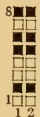
FIG. 155. these two threads can be drawn on one harness, giving the same result.
