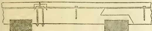
Fig. 2.—Section of sleepers, showing the joint-plates, and mode of fastening the rails.
