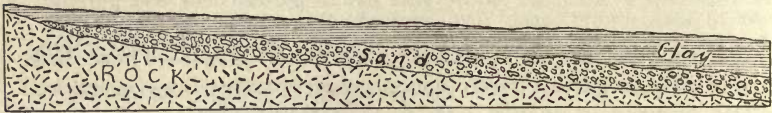
Fig. 17 Illustrates the case where an impervious bed overlaps completely the intake area of the porous bed, thus greatly diminishing or cutting off its water supply. This porous bed may be, at other points along its outcrop, bared of this impervious overlap and thus be water-bearing.
