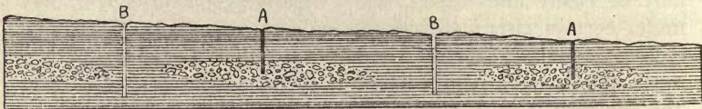
Fig. 19 Shows the case where gravelly beds of ancient streams or the beaches of ancient lakes have become buried under the later accumulations of impervious materials and rest on the same. Two of these lines of gravel, which may be narrow and sinuous but which may extend for miles, are here shown in cross section. Unlike the case represented in the preceding figure, the gravels are not completely enclosed in clays, but in other parts of their courses are bared of the impervious cover and have thus become water-bearing. Wells at AA which go down into the ancient channels would be successful, while those at B and B wholly in the impervious material would not.
