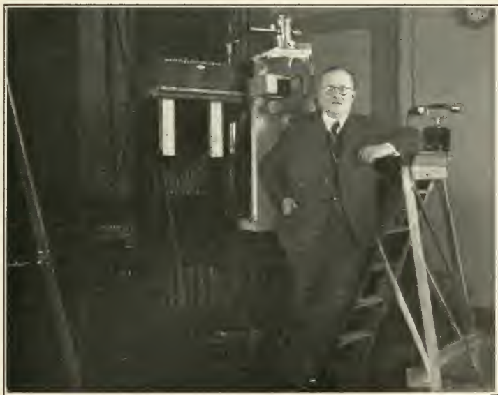
2. M. DE HAAS IN FRONT OF THE ELECTROMAGNET AND THE CRYOSTAT USED FOR ADIABATIC DEMAGNETIZATION.
