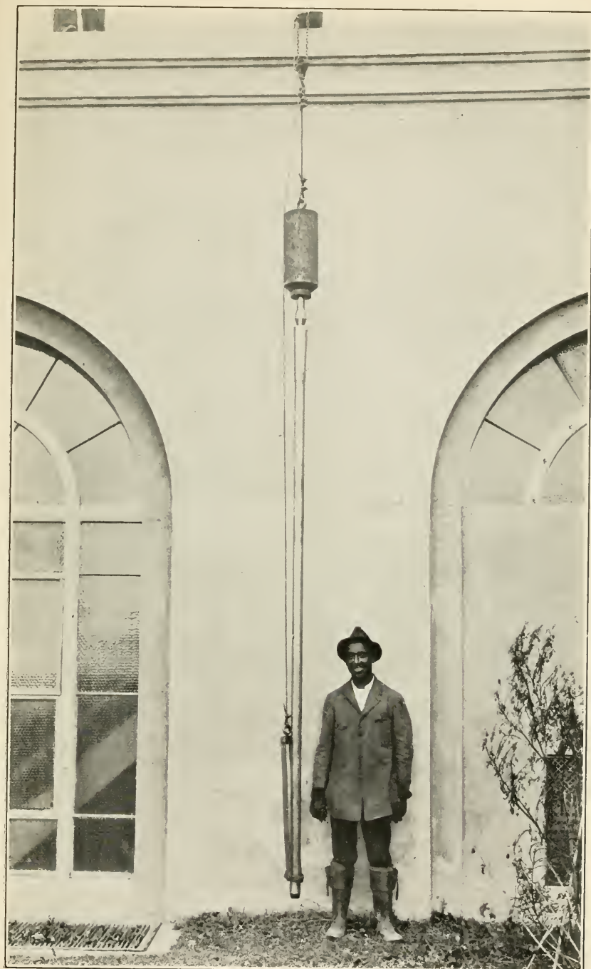
THE CORE SOUNDING APPARATUS ASSEMBLED READY TO LOWER.
