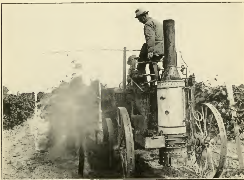
FIG. 2.—STEAM-ENGINE POWER SPRAYER USED IN SPRAYING AGAINST THE GRAPE LEAFHOPPER, NORTH EAST, PA., 1912. (ORIGINAL.)
