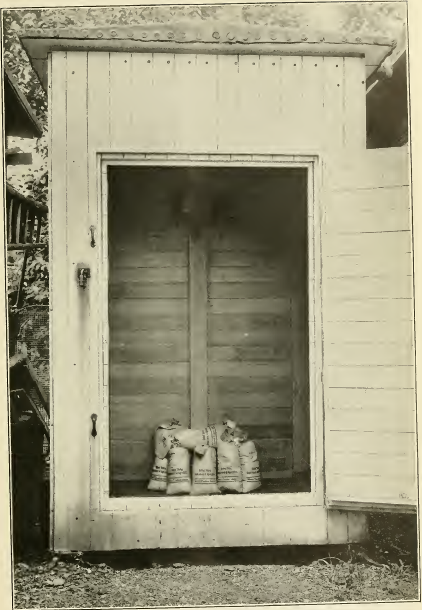
FUMIGATING BOX USED IN EXPERIMENTS WITH PARA-DICHLOROBENZENE. (ORIGINAL.)
