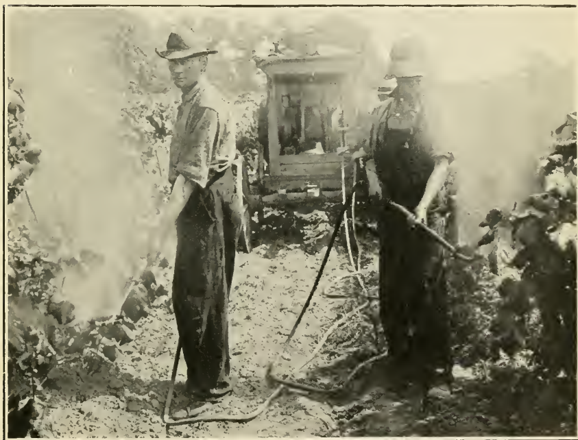
FIG. 2.—GASOLINE-ENGINE SPRAYER SUPPLYING POWER FOR TWO "TRAILER" LEADS OF HOSE IN SPRAYING AGAINST THE GRAPE LEAFHOPPER. VINEYARD OF MR. J. E. BEATTY, NORTH EAST, PA. (AUTHOR'S ILLUSTRATION.)
