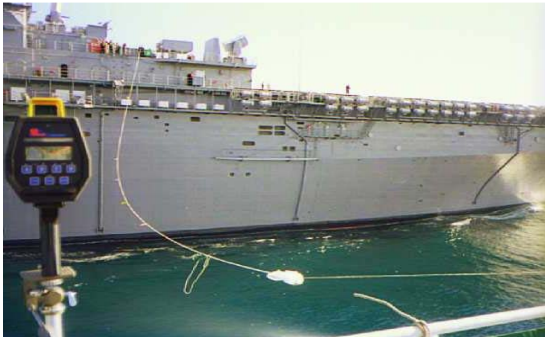
Figure 5. Twenty minutes after LHD-4 crossed the T-AO 199 stern with rangefinder providing continuous data [From Ref. 6].
