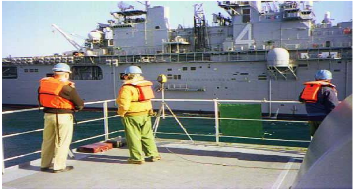
Figure 4. Rangefinder setup on forecastle with LHD-4 alongside from [Ref. 6].
