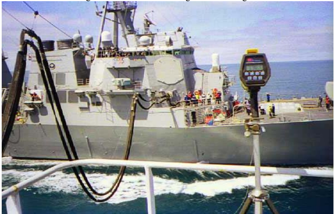
Figure 7. DDG-53 alongside with rangefinder in foreground [From Ref. 6].
