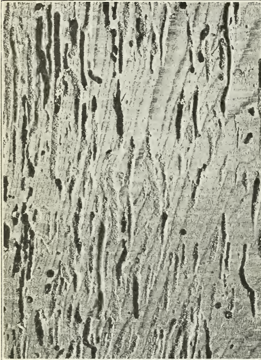
FIG. 30.—Powder-post defect in pine made by Xyletinus peltatus
