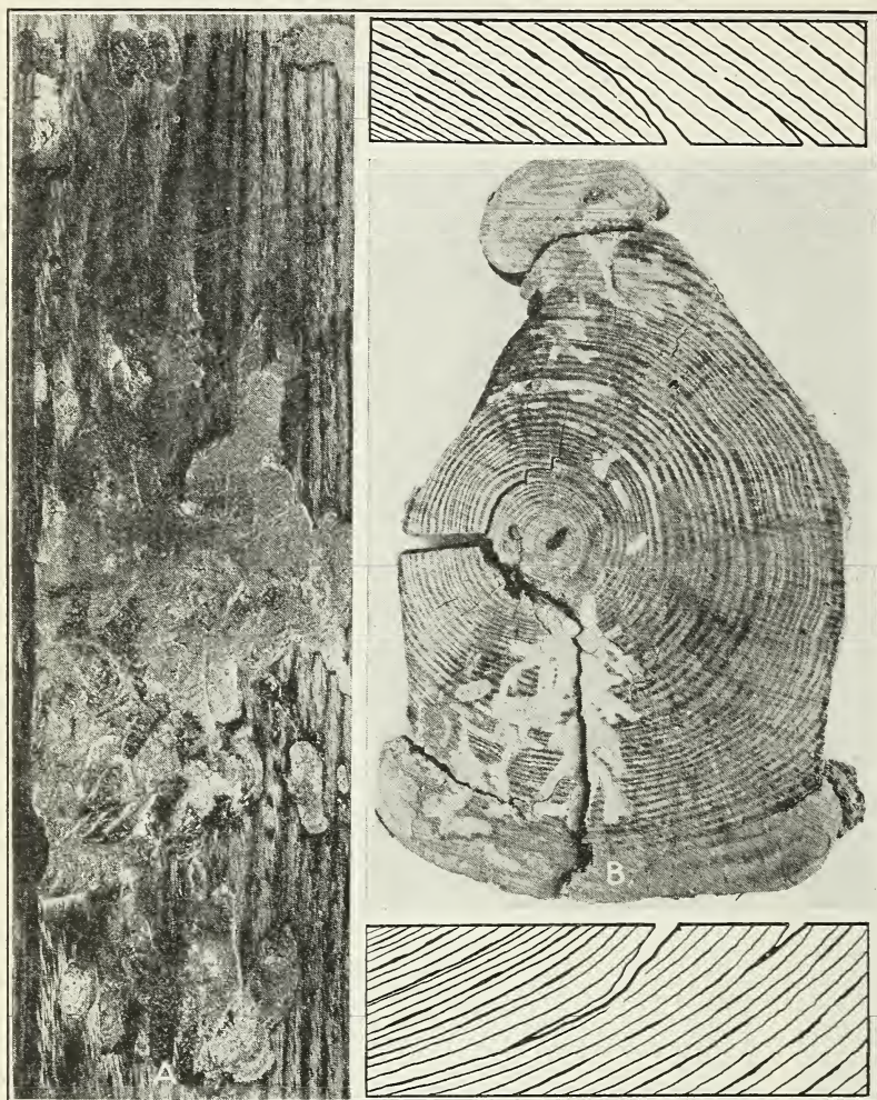
FIG. 24.—A, grub holes made by a flat-headed borer ( Buprestis apricans ) in the pitchy "fatwood" of the basal log of long-leaf pine; B, the same in a turpintined tree
