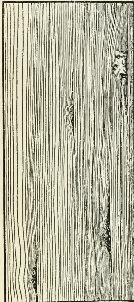
FIG. 41.—Black check in western hemlock, radial section. (6)
