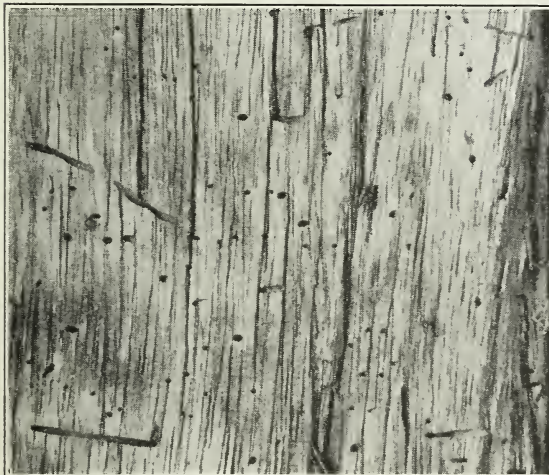
FIG. 14.—Pinhole damage by ambrosia beetles ( Xyleborus grenadensis ) to Hura wood (Rakuda) imported from Central America
