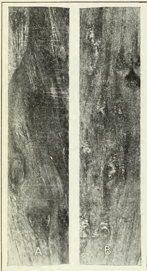
FIG. 29.—A and B, two views showing small "pitch pocket" or "bird's eye," caused by larva of a fly in western yellow pine
