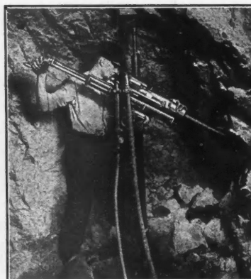
CP-5W Mounted Drifter, Wet, speeding-up drilling for the United Mine Company, Oatman, Arizona. High cutting speed in various formations is assured by rapid, powerful blows with strong rotation. Weight 112 pounds. Economical drilling depth, 8-12 feet.
