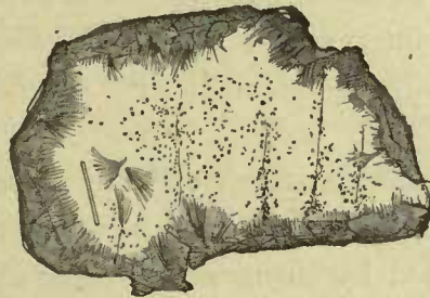
FIG. 4. Clastic quartz partially converted to serpentine, which penetrates from the outside in needles. The specks within the quartz are fluid inclusions and the straight prism is a small apatite. Magnified 53 diameters.
