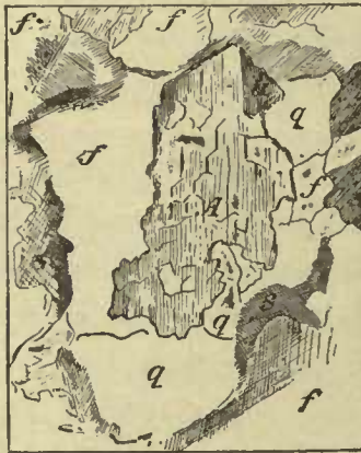
FIG. 2. Authigenetic augite in altered sandstone, No. 8, Coast Ranges. A, augite; u, uralite; f, microcrystalline feldspar; q, quartz grain; s, serpentine. Magnified 117 diameters.
