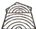
Fig. 2. The end of a typical wooden coffin. The lid and the box are each carved out of a single tree. The ends are sawn off smooth.
