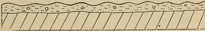
FIG. 2. Cross section illustrating furrowed-floor type of sheet-flow. Bedrock below with fine detritus containing occasional pebbles above.
