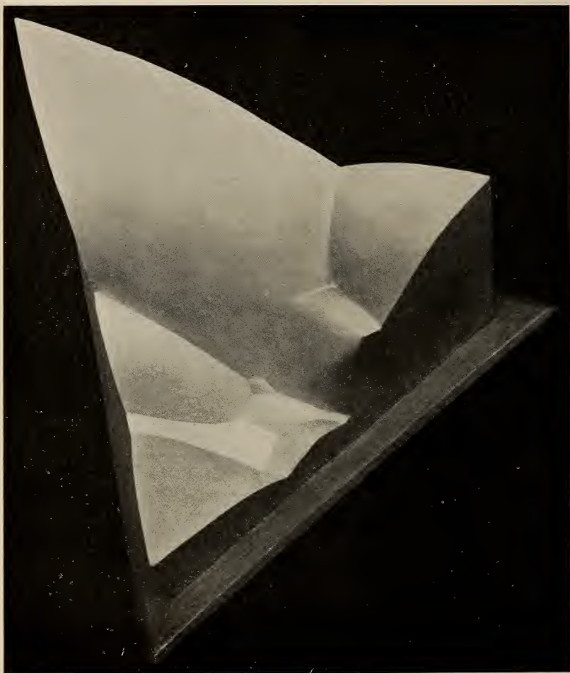
FIG. 11.—The complete temperature concentration diagram which was constructed by plotting vertically upon the concentration diagram given in fig. 8 the temperatures of complete fusion of the various compositions.
