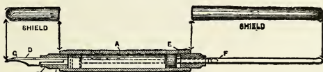
A, Barrel; B, Nozzle; C, Pen; D, Feed; E, Plunger; F, Rod.
