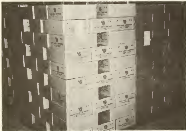
Figure 2. Pallet load with partial provision for air flow through the stack
