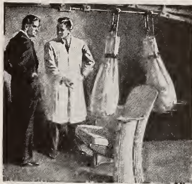
"Swinging impact" tests assure maximum durability for chair backs, back fastenings to standards, and floor anchorage.
