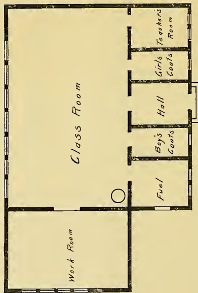
PLANS FOR REMODELING OLD BUILDING.—Class room inside measurement 32x22; work room 22x12; fuel room 8x8; boys' and girls' coat rooms 5x8; hall 6x8; teachers' room and supplies 8x8.
