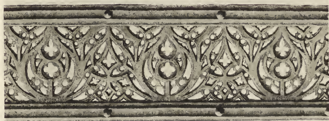
FIG. 38. THE TWO PLATES RIVETED TOGETHER.
