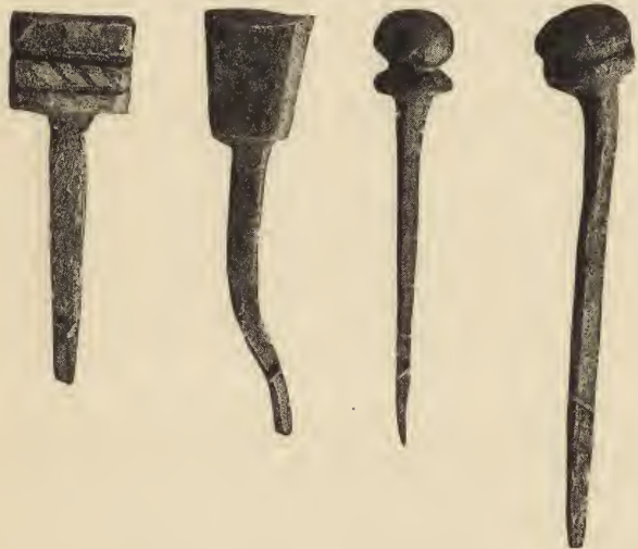
FIG. 5. IRON NAILS WITH WROUGHT HEADS.
