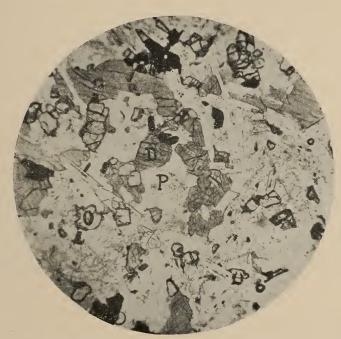
FIG. 4.—Photomicrograph of Railroad Mountain dike. 50 X. Showing diallage (D), olivine (O), and magnetite (opaque) in a matrix of interlocking plagioclase crystals (P).
