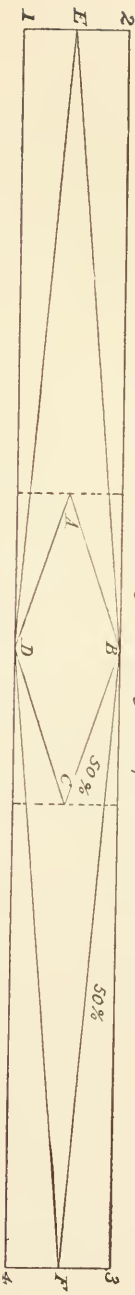
Fig. 1. Vessels of equal coefficients may have very unequal fineness of form.
