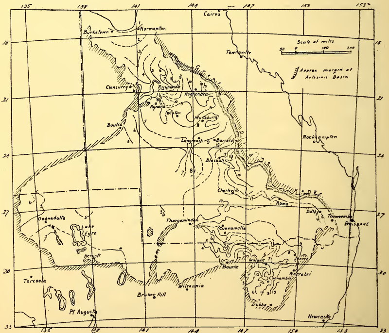
Diagram IV.—ISOPOTENTIALS FOR 1912; the figures represent hundreds of feet above sea-level.
