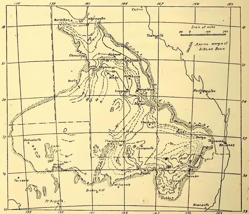
Diagram I.—CONTOURS OVER FLOOR OF BASIN; figures in hundreds of feet below sea-level.
