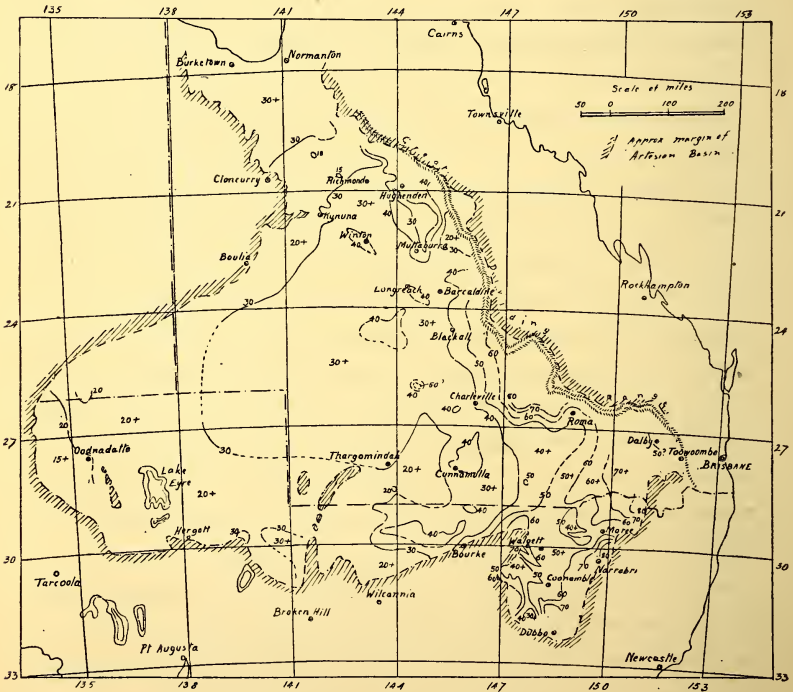
Diagram II.—AREAL DISTRIBUTION OF TEMPERATURE GRADIENTS; figures represent values in feet per degree F. (20+ indicates 1° F. for 20 - 29 feet; 30+, 1° F. for 30 - 39 feet, etc.).
