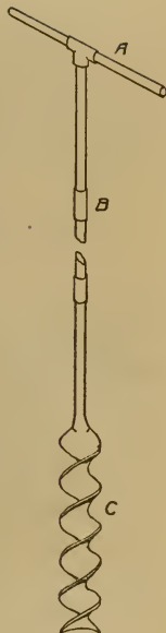
FIG. 1. — Auger for taking soil samples. (A) handle, (B) joint, (C) worm with modified cutting edge.
