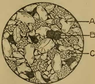
FIG. 6. — Structure of a loam soil in good tilth. (A) sand particle, (B) pore space, (C) granule composed of silt and clay particles.
