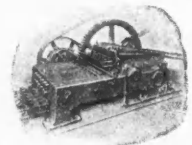
NO. 1 WHITE BRIQUETTING PRESS, CAPACITY 100 TONS IN 10 HOURS. BUILT IN 3 SIZES.
