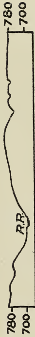
FIG. 4. Cross-section of Rock River Valley about 3 miles below the mouth of Kishwaukee River. The numbers at the ends represent elevation above the sea. R. R. = Rock River. Length of section a little more than 3 miles. Vertical scale exaggerated about 8½ times.
