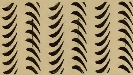
FIG. 24. — Element of the Parsons Turbine.
