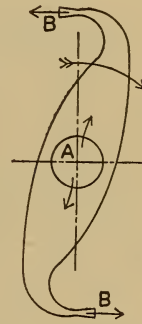
FIG. 17. — Outline of an Elementary Reaction Wheel.
