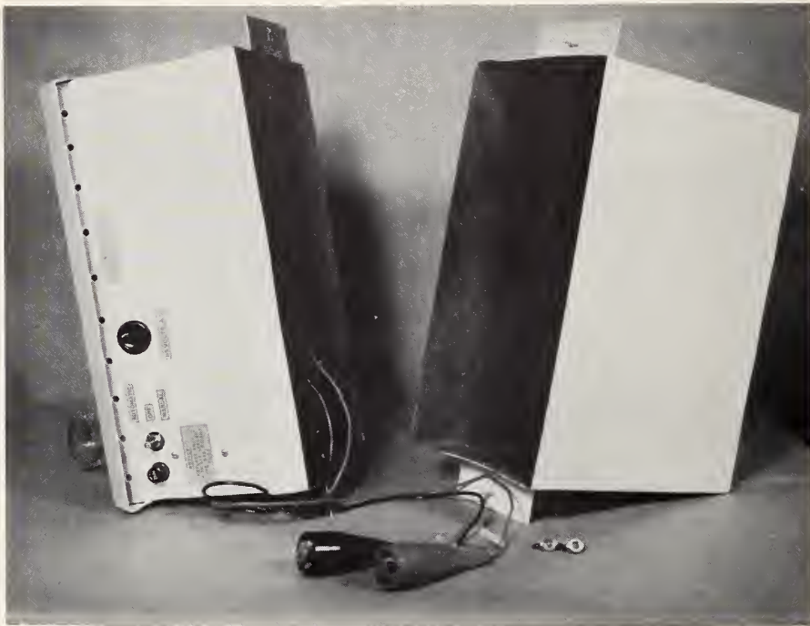
Figure 7.--Complete power supply with cover removed from battery case.
