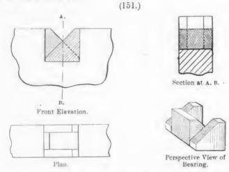
The Board of Trade have examined and tested a pattern of price computing weighing instrument, similar in principle of construction to the one referred to in Notice 90, dated November, 1909 (see p. 620 of the "Board of Trade Journal" of 30th December, 1909), but provided with new pattern bearings as herewith shown; and have issued a certificate (No. 112) under the provisions of Section 6 of the above Act that the pattern is not such as to facilitate the perpetration of fraud.
