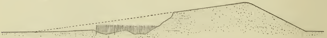
FIG. 8.—Repairing a larger breach by means of sand fences. The diagram represents a cross section of a dune with two rows of sand fence parallel to the dune and cross rows extending from the outer row to the broken face.
