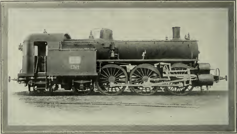
4-CYLINDER EXPRESS-COMPOUND, SOUTHERN RAILWAYS OF ITALY.
