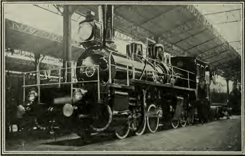
THE MOST POWERFUL ENGINE EXHIBITED AT PARIS—THE TWELVE-WHEEL COMPOUND OF THE MOSCOW-KAZAN RAILWAY.
