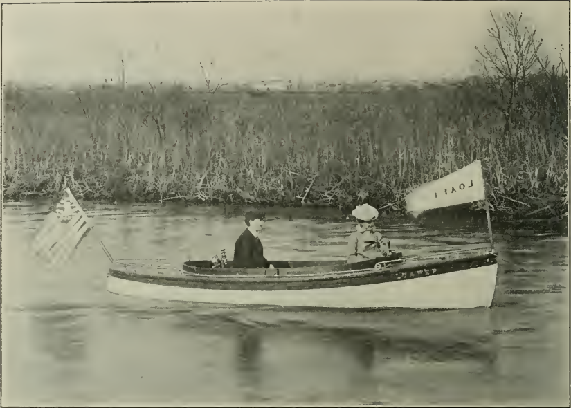
17-FOOT "TORPEDO-STERN" LAUNCH, 1\frac{1}{2} -HORSE-POWER. Truscott Boat Manufacturing Co.
