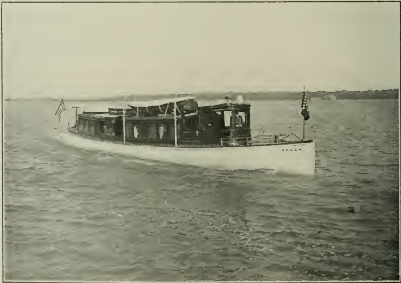
YACHT HELEN, 60 FEET BY 9\frac{1}{2} FEET, SPEED 13\frac{1}{2} MILES PER HOUR. Two 20-horse-power two-cylinder two-cycle Sintz vapor engines. Michigan Yacht & Power Co.
