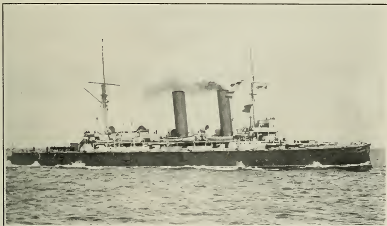
H. M. S. BLAKE—PROTECTED CRUISER, I CLASS, 20,000 HORSE POWER, 21 KNOTS.
