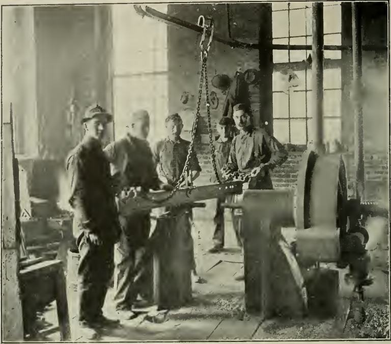
FIXED-TYPE RIVETER AT WORK.
