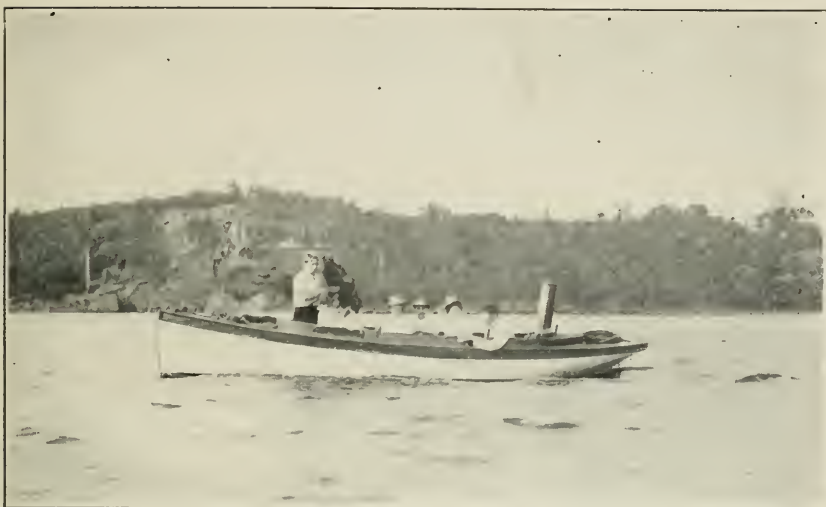
25-FOOT 4-HORSE-POWER OPEN NAPHTHA LAUNCH.
