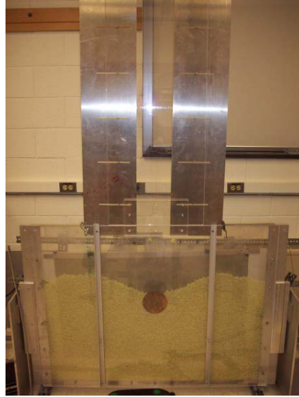
Figure 9. Bronze intruder impacting into a 2D photoelastic granular material. Experimental device built by Clark to investigate the microscopic grain-grain interactions controlling the forces affecting the intruder throughout its trajectory. The intruder is dropped from various heights translating into specific intruder impact velocities. Adapted from [6], [8].
