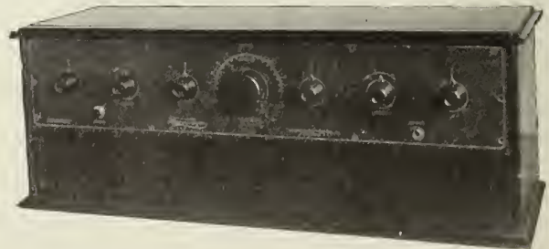
Here is the "Thermiodyne," the new six-tube wonder set manufactured by the Shepard-Potter Company of Plattsburg, N. Y. The feature of the Thermiodyne is its simplicity of control, all tuning on the entire six tubes being manipulated by the one control in the center. Great demand for the Thermiodyne is reported by the manufacturer.
