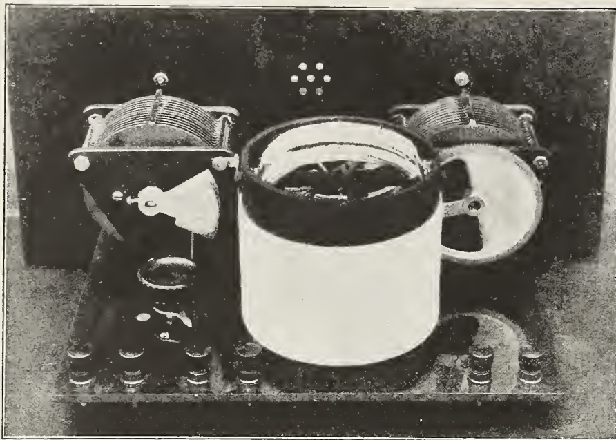
From the rear. The sub-panel simplifies the mounting, and it's fastened to the socket. It supports the coil, rheostat and binding posts, besides the wiring underneath it. Note the geared and counterbalanced type of condenser.
