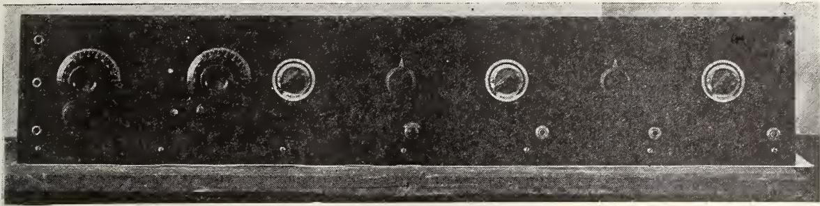
This figure shows the panel arrangement for separate control of each of the fundamental circuits. Instead of complicating matters, this control system actually makes the operation of the set much simpler.
