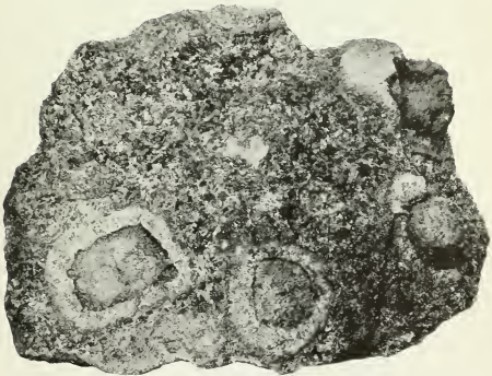
Specimens of nodule-bearing peridotite from forty-foot dike cutting schistose rocks of Basic Complex. The nodules are granular aggregates of olivine, regularly surrounded with kelyphitic shells, as shown. Two-thirds natural size.
