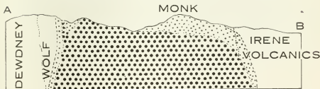
FIGURE 21.—Section along line A-B of figure 20, on the same scale; illustrating explanation of great breadth of metamorphic aureole southeast of larger granite stock. Apophysal dikes in roof of stock not shown.
